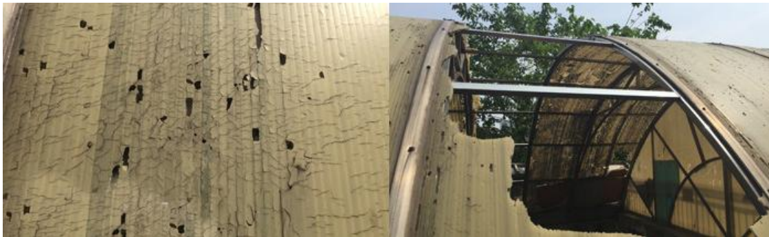
After using PC endurance boards made from recycled materials for a period of time
